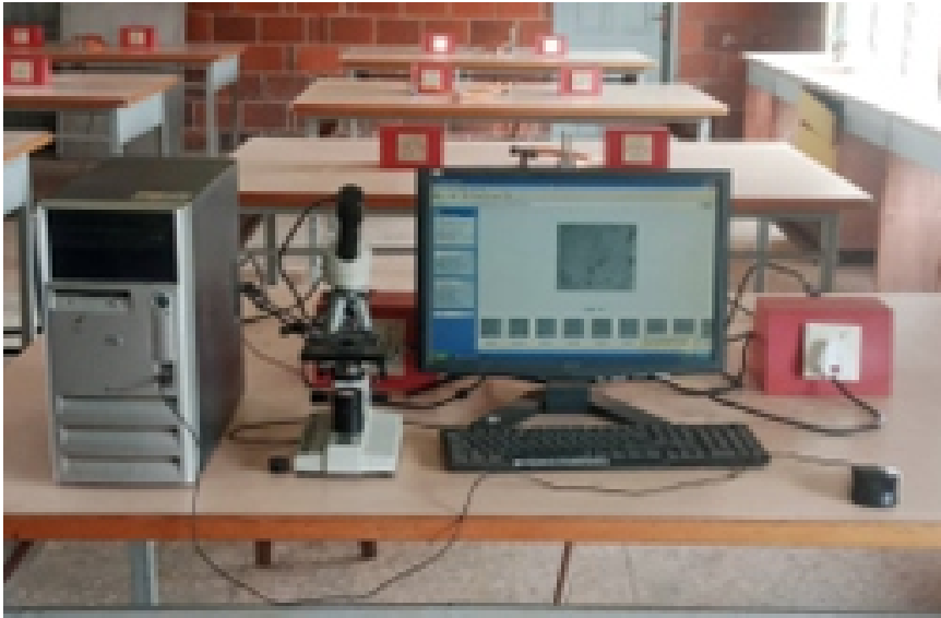
Radon analysis Lab Ota: High-quality mono-chrome charge coupled device (CCD) TV camera connected to a PC-based image analyzer (Image-Pro Plus version 4.0) and computer.
